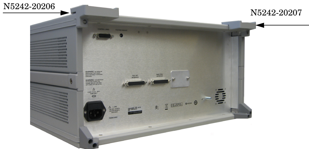
Figure 7 Install Locking Feet on Test Set
